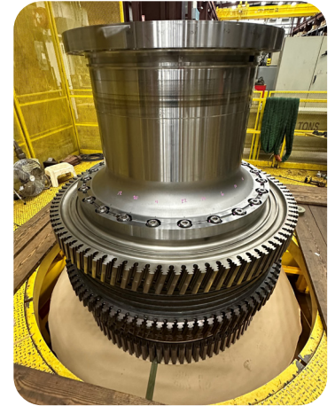
TURBINE ROTOR IN STACK
