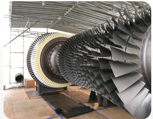
SEED ROTOR INSTALLED WITH NEW ROW 9-17 COMPRESSOR WHEELS
