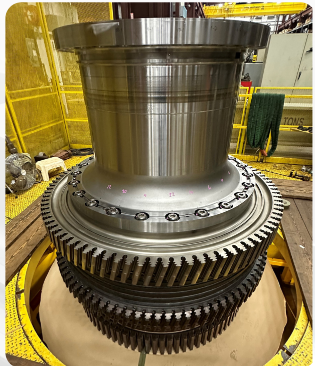
TURBINE ROTOR IN STACK
