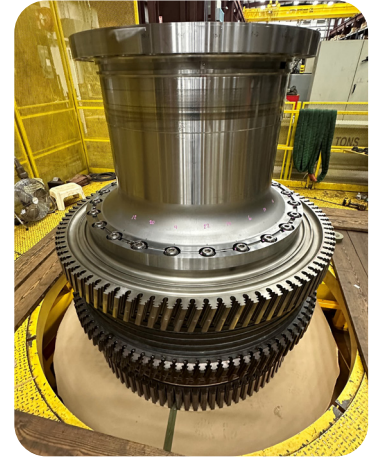
TURBINE ROTOR IN STACK
