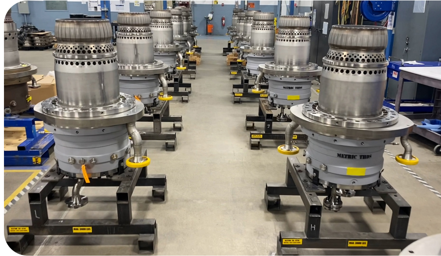
FLAMESHEET™ PRODUCTION LINE - EACH UNIT IS TESTED PRIOR TO SHIPMENT
