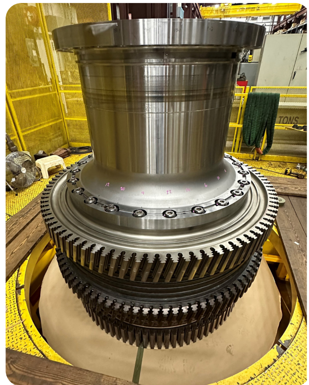
TURBINE ROTOR IN STACK
