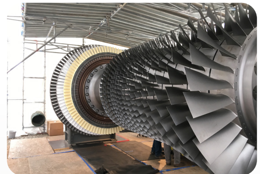
PSM SEED ROTOR INSTALLED WITH NEW ROW 9-17 COMPRESSOR WHEELS
